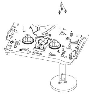
Fig.3-18 CAPSTAN MOTOR REMOVAL
